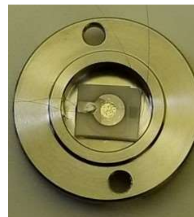
b) Diamond detector on the detector cap
