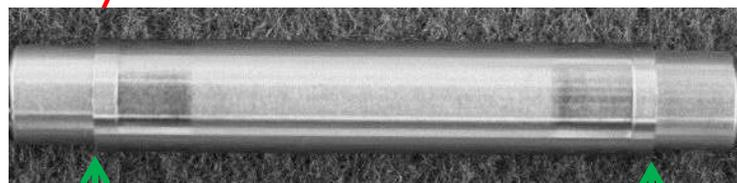
加圧抵抗溶接(PRW: Pressurized Resistance Welding)
